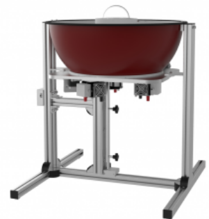
Fig. 2: Open integrating sphere with transparent dome
