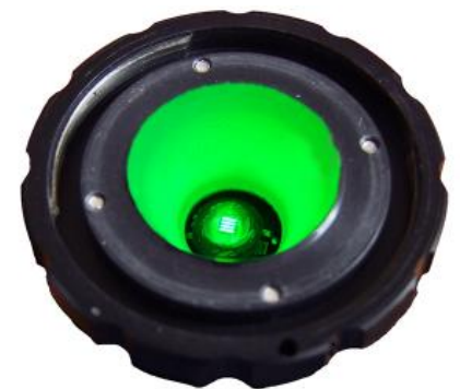
The conical measurement port is placed over the test LED and detects all the radiation in a 2pi space
